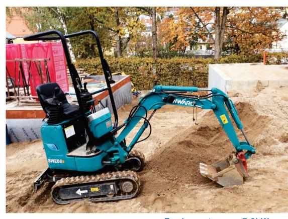
Engine netpower:7.2kW Machine weight:1010kg
